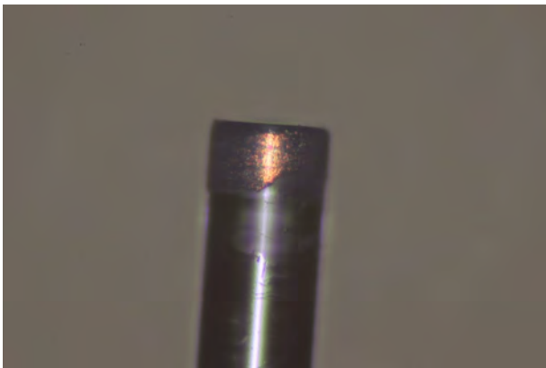
Bright-field image of a fiber-mirror. Courtesy of OMT fellow Irene, UKON.
